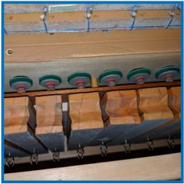
These are some of the 58 pneumatic motors on the Swell Organ which control the wind to each individual pipe as a key is depressed. The brown leatherwork near the bottom of the picture had begun to perish allowing air to escape. This leatherwork dated back either to the cleaning and overhaul of the organ in 1989 or the rebuild of the organ in 1965.
